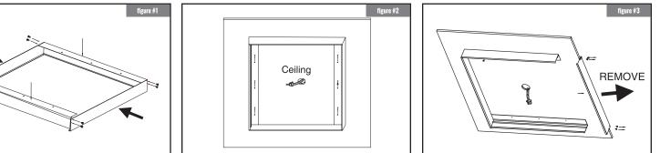
1. Assemble the mounting frame with the 8 screws(included)
