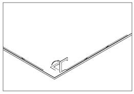
1. Pull earthquake clip away from panel until facing perpendicular to the panel surface.
